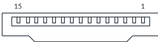
Figure A-14: MIPI CSI 2-lane connectors
